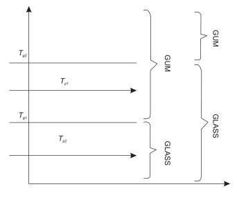
FIGURE. 1. The influence of product temperature  $(T_p)$  and glass transition temperature  $(T_s)$  on the state of material during spray drying (*descriptions in the text*) [Samborska *et al.*, 2011].
