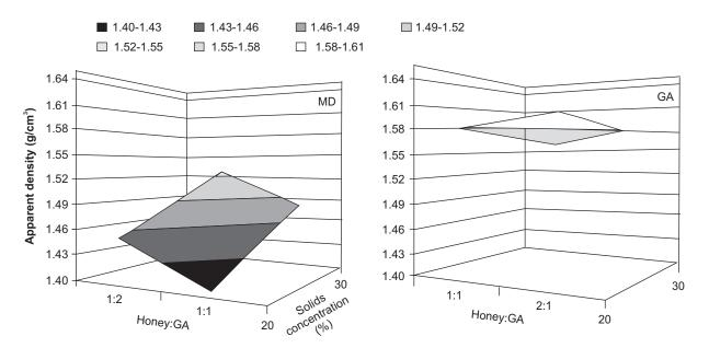
FIGURE 3. Surface plot showing the effect of honey content and solids concentration on apparent density (g/cm<sup>3</sup>) of powders obtained after spray drying of honey solution with maltodextrin (MD) and gum Arabic (GA).
